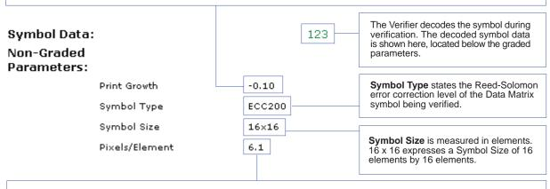
For consistent and reliable verification, a symbol must have a minimum of 10 **Pixels Per Element** (PPE). Pixels Per Element refers to the number of pixels in the **width** of each individual symbol element. The Verifier appends a Pixels Per Element value to ISO/IEC 15415 verification reports.
